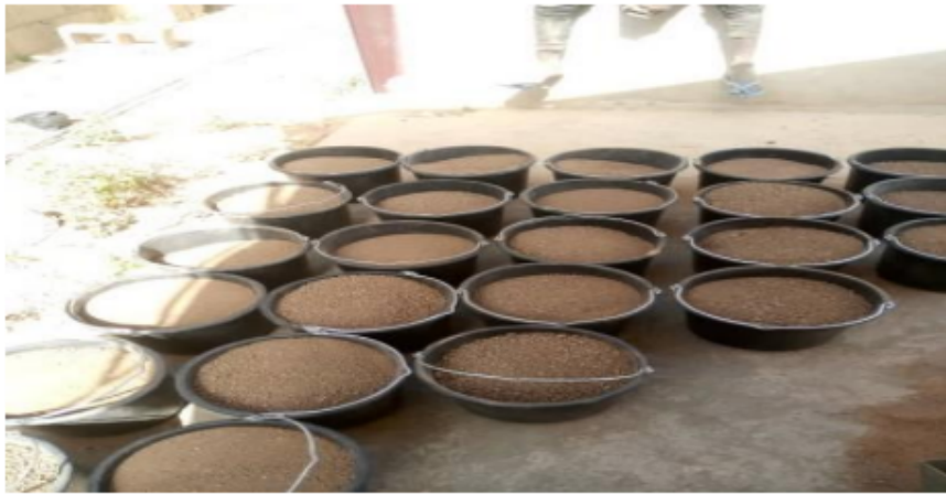
Picture 2: Soil proportioning for mixing
