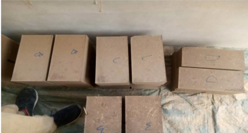
Picture 3: Compressed stabilised mud brick samples
